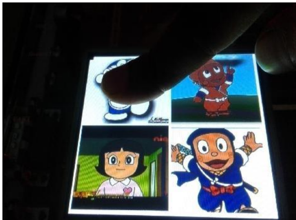
Fig- 12 GLCD display shows that the player touched one of the four images while playing a game.
