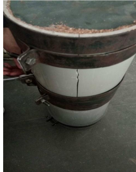
Fig. 4 Failure Pattern of the sand pile
