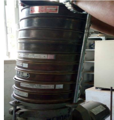
Fig.1 grain size determination by sieve analysis
