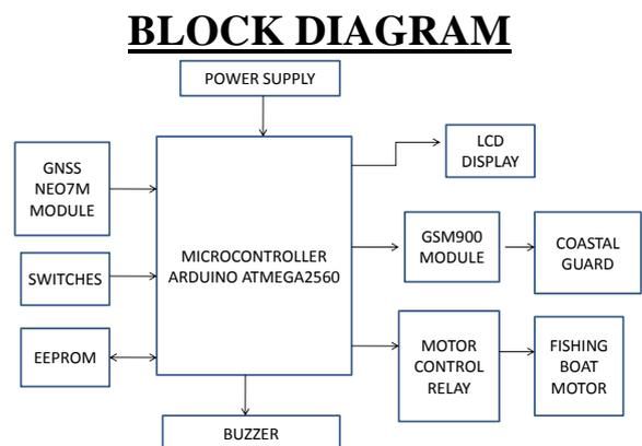
In this Project it is proposed to design an embedded system which is used for tracking and positioning of any vehicle by using Global Navigation Satellite System (GNSS) and Global system for mobile communication (GSM).
