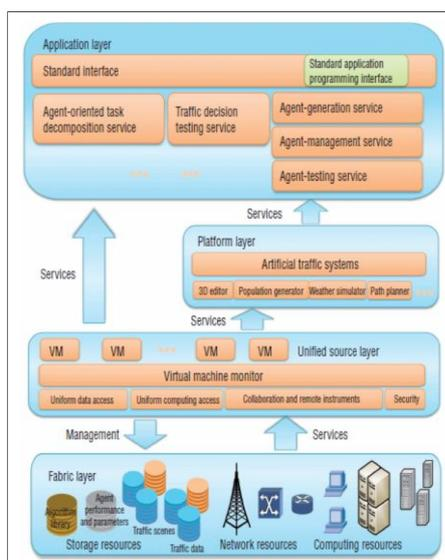
**Fig-2:** Intelligent traffic clouds structure has application, platform, unified source, and fabric layers.
