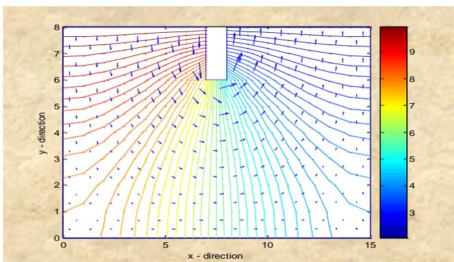
Figure 4.1: Equipotential lines and streamlines under a dam
