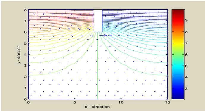
Figure 4.4: Equipotential lines and stream lines for  $K_x \geq K_y$
