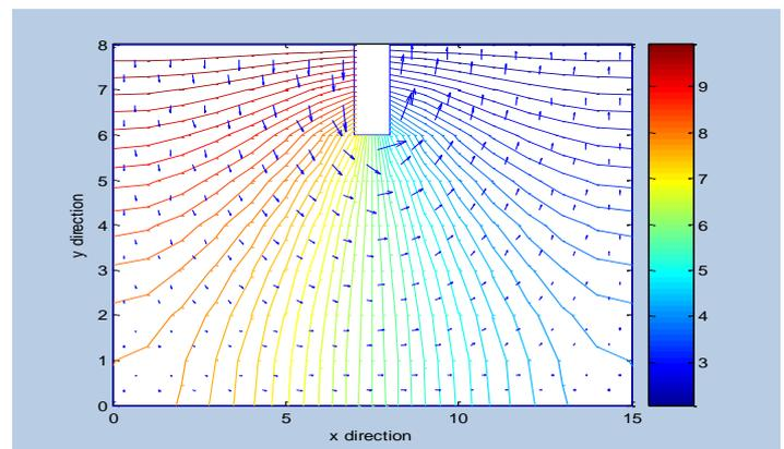
Figure 4.2: Equipotential lines and streamlines for  $K_x = K_y = 200 \text{ m}^3/\text{day}$ .
