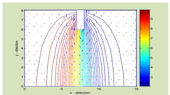
Figure 4.3: Equipotential lines and stream lines for  $K_x \leq K_y$
