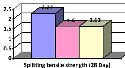
0% Coconut shell 5% Coconut shell 10% Coconut shell
