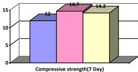
0% Coconut shell 5% Coconut shell 10% Coconut shell
