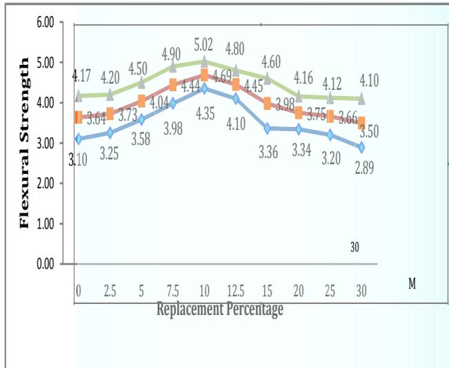
Graph:- 5 Flexural Strength in N/mm<sup>2</sup> at 28 Days
