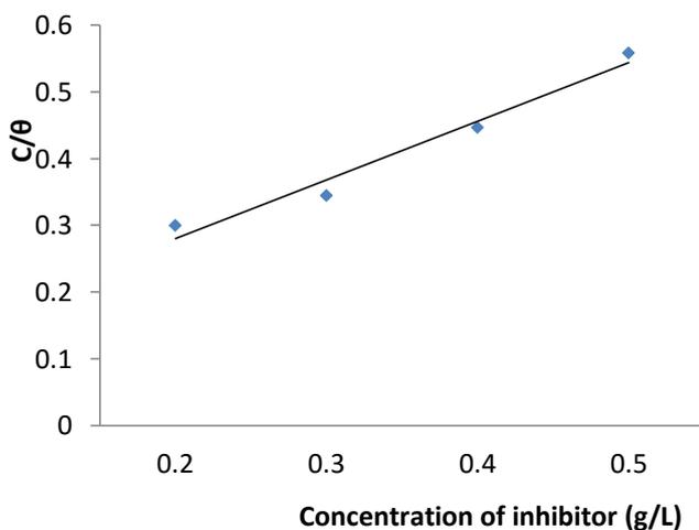
**Figure 4:** Langmuir isotherm for *Terminalia ivorensis* adsorption on Aluminium alloy AA8011A in 0.5 M HCl
