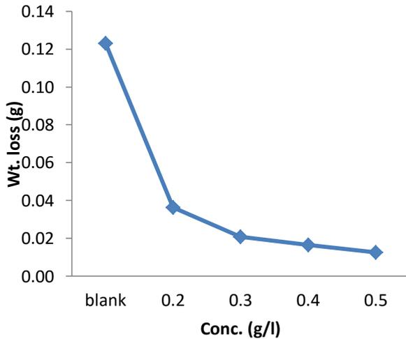
**Figure 2:** A plot of weight loss (g) of various concentrations of *Terminalia ivorensis* in 0.5 M HCl on mild steel
