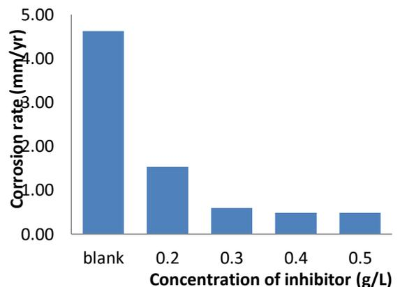
**Figure 1:** A plot of Corrosion rate of various concentrations of *Terminalia ivorensis* in 0.5 M HCl on mild steel
