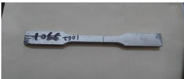
Fig.3: Specimen before subjecting to tensile test
