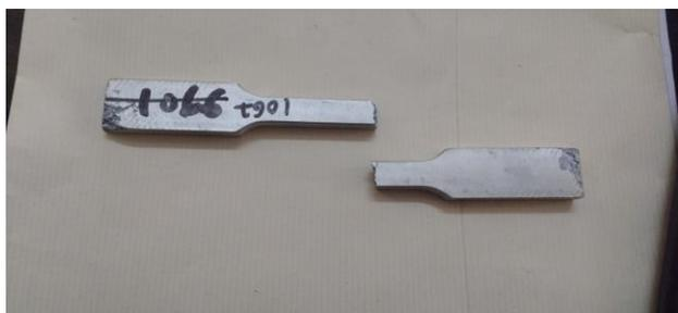
Fig.4: Specimen after subjected to tensile test
