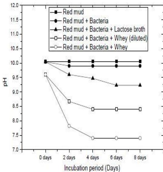
**Figure 8 Dissimilarity of pH value of red mud under different conditions**
