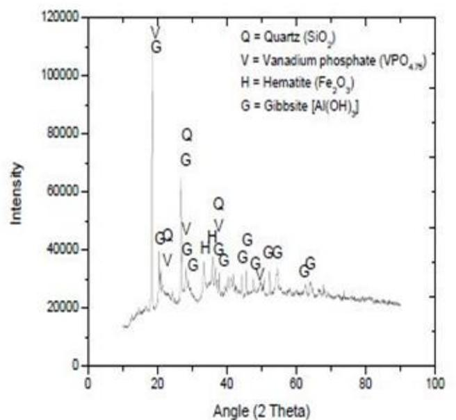
**Figure 10 XRD analysis of bio-neutralised red mud**
