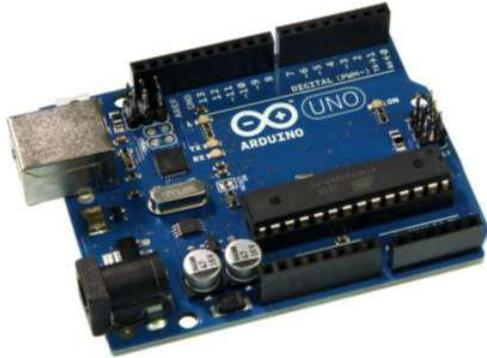
**Fig-7:** Arduino Microcontroller
