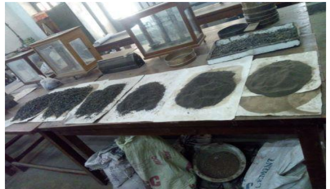
Figure 1 Gradation of aggregate sample
