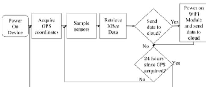
The diagram shows the high level software block for a single environmental data collection device. The microcontroller is programmed in C using MPLAB XC32, an integrated development environment built by Microchip Technology.
