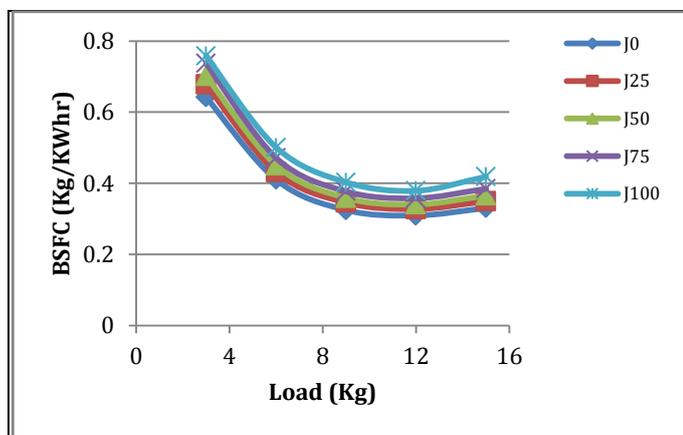
Figure 6 Variation of BSFC (Kg/KW hr) with load (Kg)
