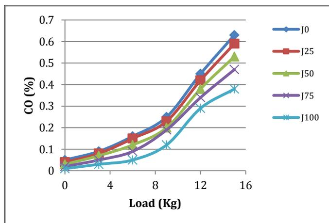
Figure 8 Variation of CO emission (%) with load (Kg)
