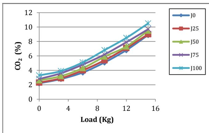
Figure 10 CO<sub>2</sub> emission (%) variation with loading (Kg)
