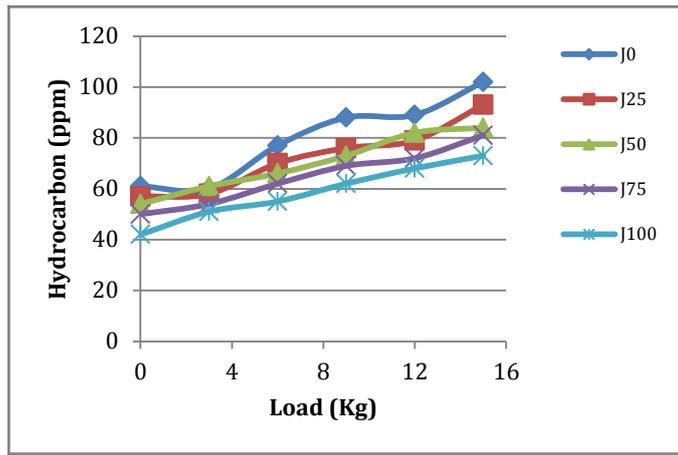
Figure 9 Variation of HC emission (ppm) with the load (Kg)
