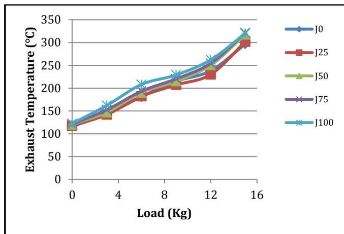
Figure 7 Exhaust gas temperature (°C) variation with loading (Kg)
