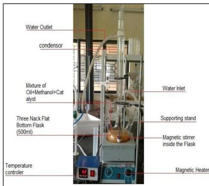
Fig. 3 Transesterification Apparatus
