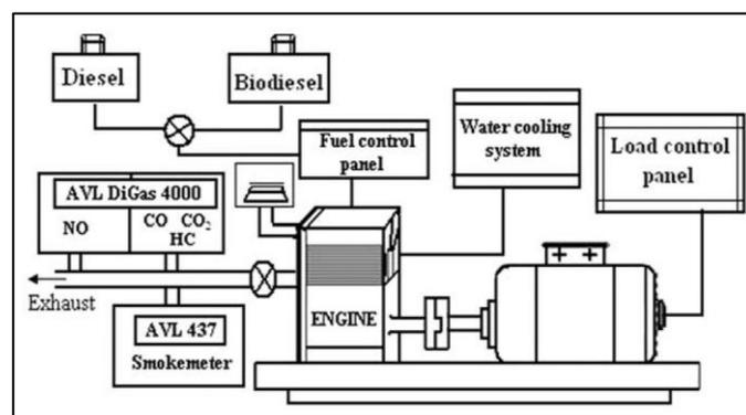
Fig. 4 Schematic diagram of the Experimental Engine setup
