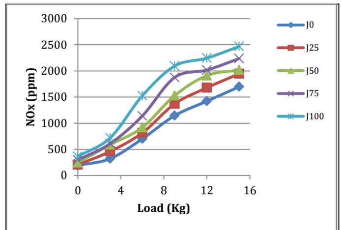
Figure 11 Variation of NO<sub>x</sub> (ppm) with load (Kg)
