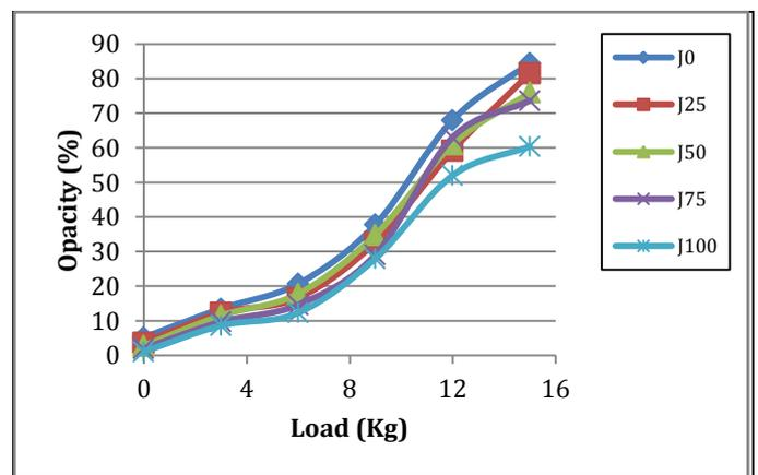
Figure 12 Variation of the smoke opacity (%) with load (Kg)
