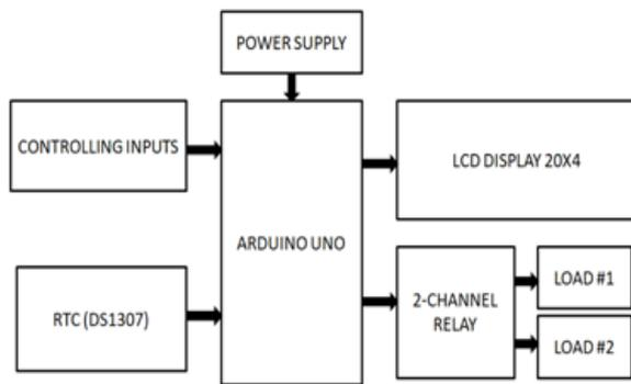
Figure 5: Block diagram
