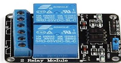
Figure 4: Relay module
