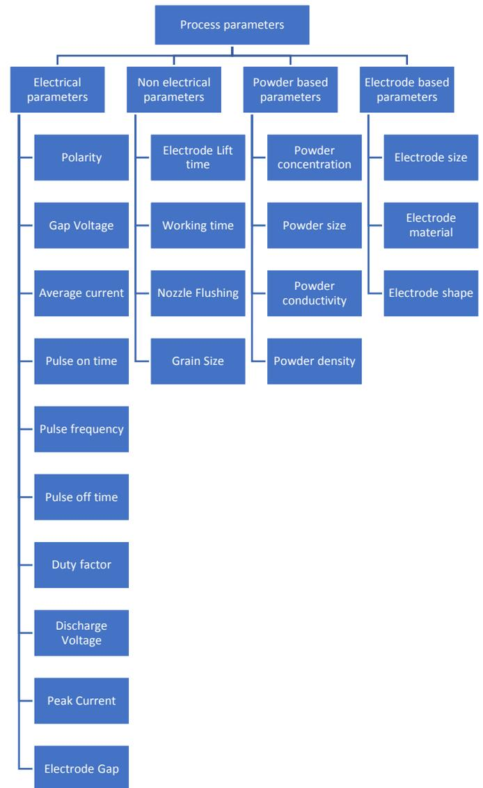
Fig -4. Major EDM Process Parameters
