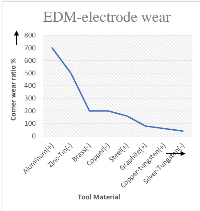
Fig -3. Electrode Wear Ratio with respective tool material
