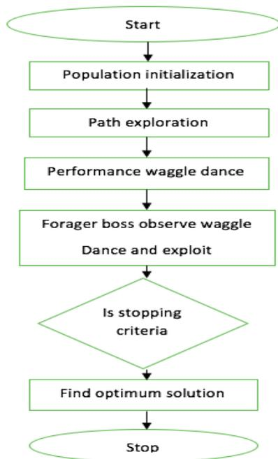
Fig -8. Procedure of Bee Colony Optimization
