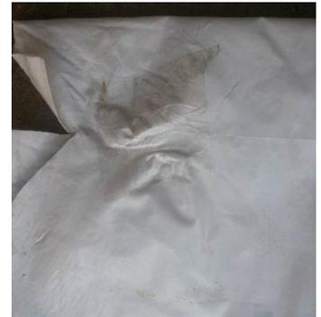
Fig - 1: LD bag, SABIC, Saudi Arabia and snap of bag which has a hole
