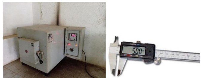
Figure -7: Test setup for the determination of Coefficient of thermal expansion capacity
