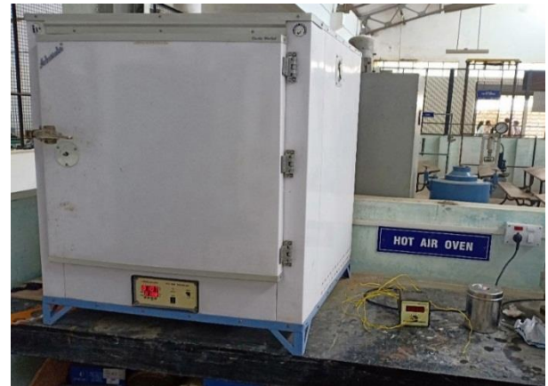
Figure -6: Test setup for the determination of specific heat capacity
