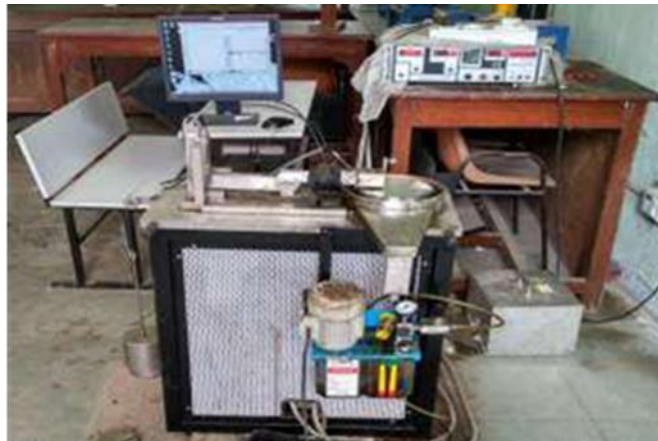
Figure 6: Schematic Setup of Pin ON Disc Machine
