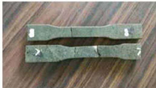
Fig: After Tensile Test specimen
