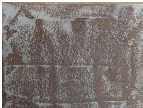
Fig: 70 % epoxy resin + 30 % (groundnut shell and rice husk)
