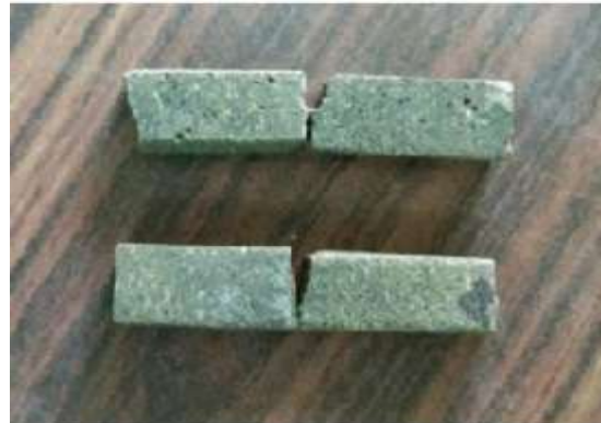
Fig: After Impact Test specimen
