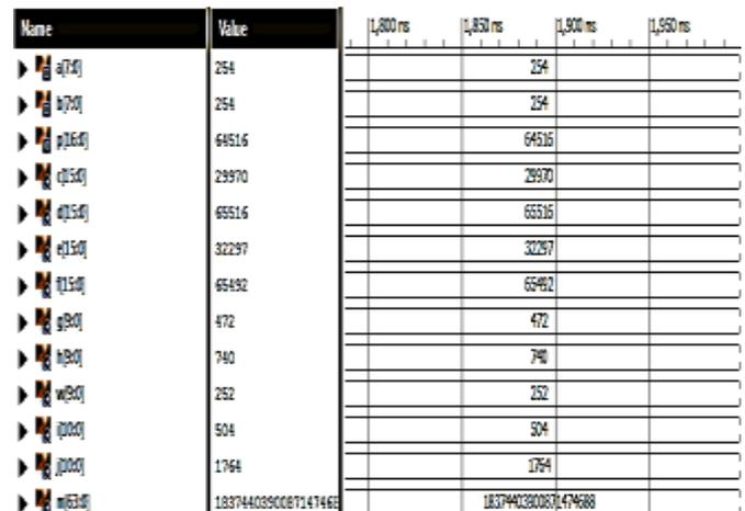
**Fig-6:** Simulation results of 8x8 Wallace multiplier by RCA
