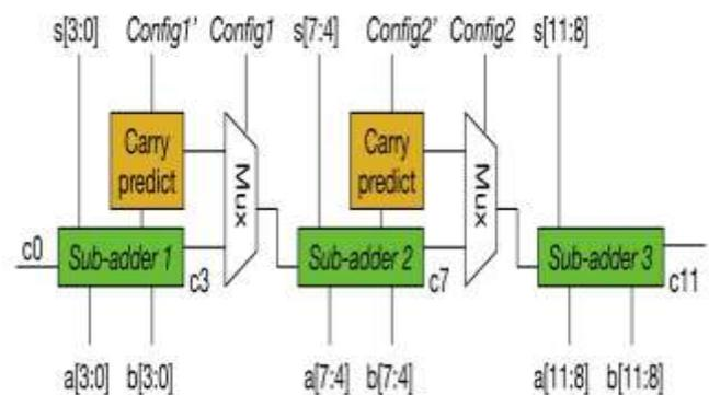
Fig-1: Carry-prediction-based configurable adder.
