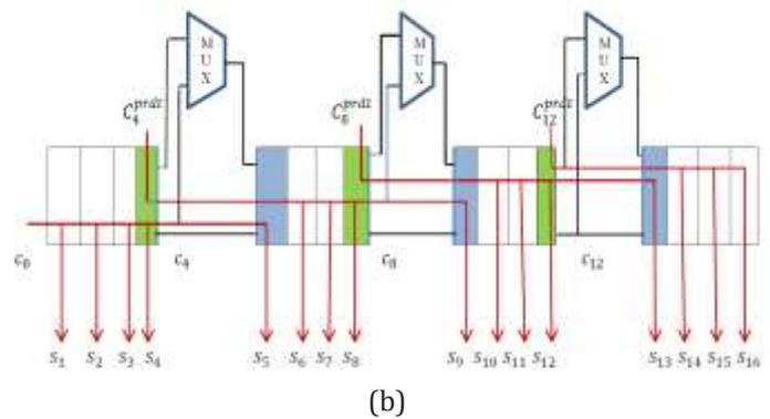
Fig-4: Implementation of 16-bit adder in (a) RCA and (b) SARA.
