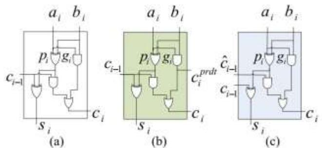
Fig-2: (a) Conventional full adder. (b) Carry-out selectable full adder. (c) Carry-in configurable full adder.
