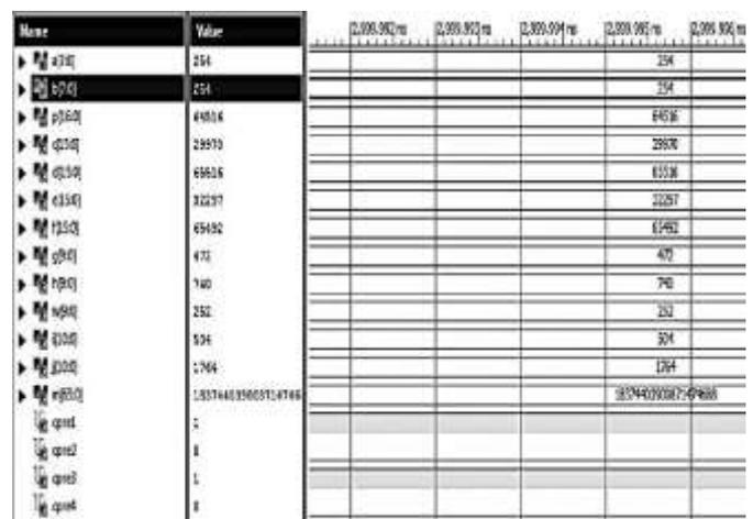
**Fig-7:** Simulation results of 8x8 Wallace multiplier by SARA
