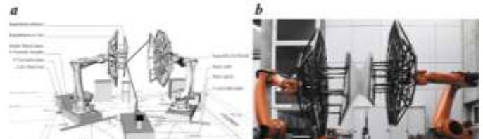
Fig -12: Schematic diagram of 12-axis robotic machine setup: (a) 3D design prototype; (b) realized design prototype [29]
