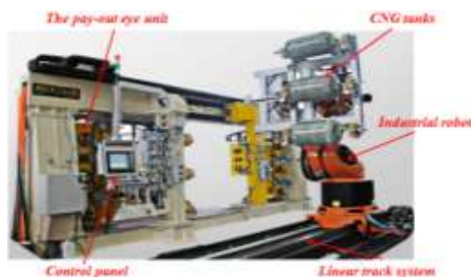
Fig -10: Filament winding machine with ind (Source: http://mikrosam.com )
