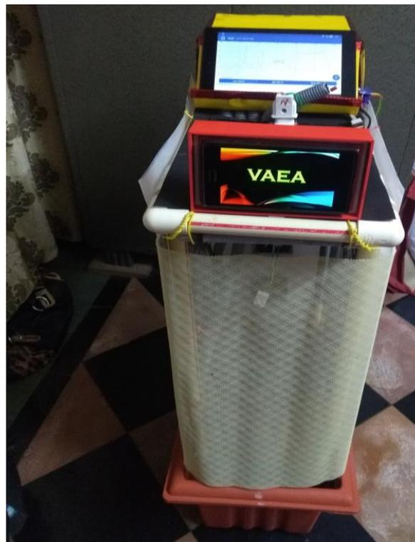
The surrounding mesh acts as a layer in isolating the inside environment of the system to the outdoor environment. A plastic cover can also be used as an alternative.
