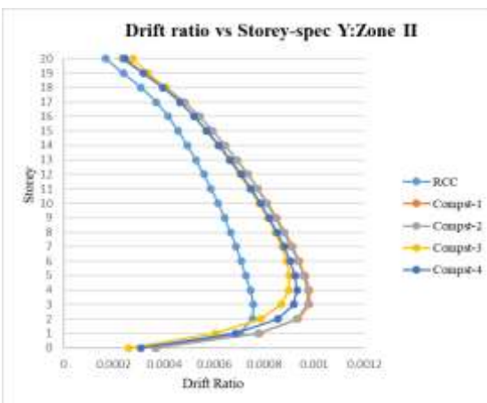
Fig -26: Drift ratio vs story along Spec-Y direction for zone II
