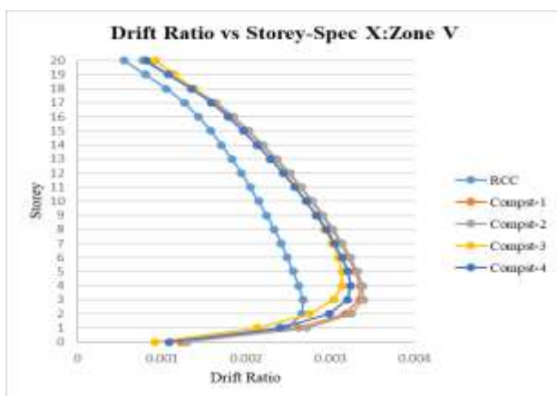
Fig -27: Drift ratio vs story along Spec-X direction for zone V
