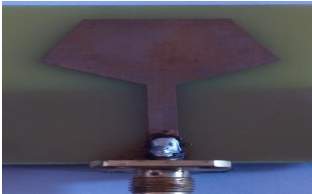
Fig-9: Fabricated antenna structure
