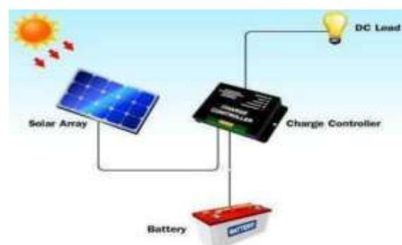
**Figure 1: Simple Block Diagram showing major components**
