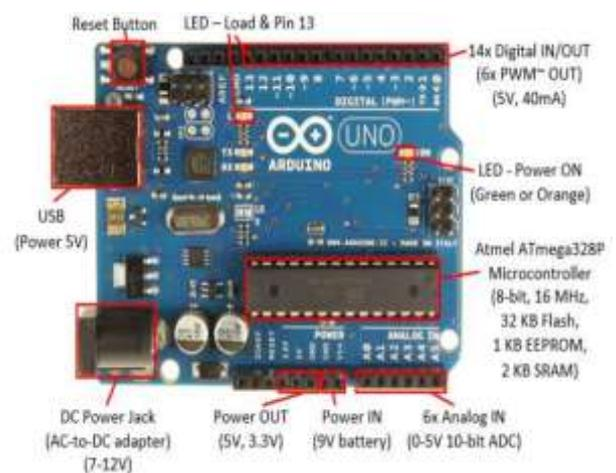
**Figure 2: Arduino uno based on ATmega328P**
