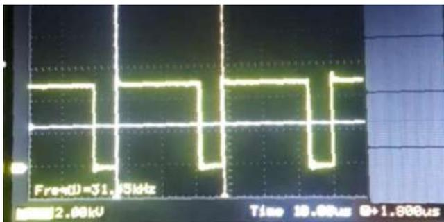
**Figure 12: The output waveform of MPPT charging**
