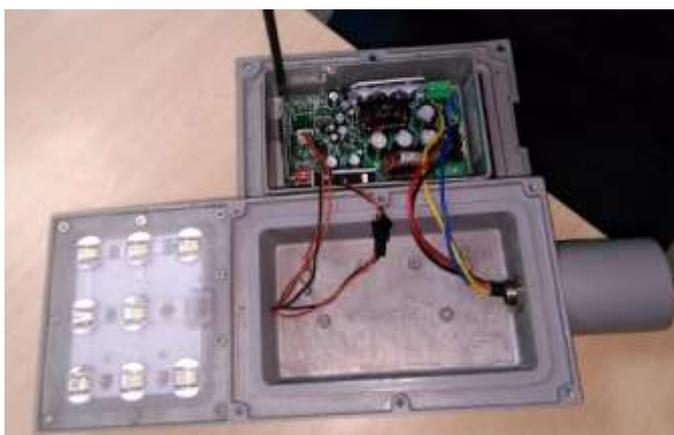
Figure 11: PCB connections to the LED panel
