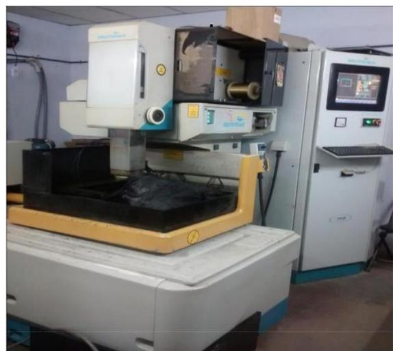
**Figure 3.1: Sprintcut Wire Cut EDM.**
