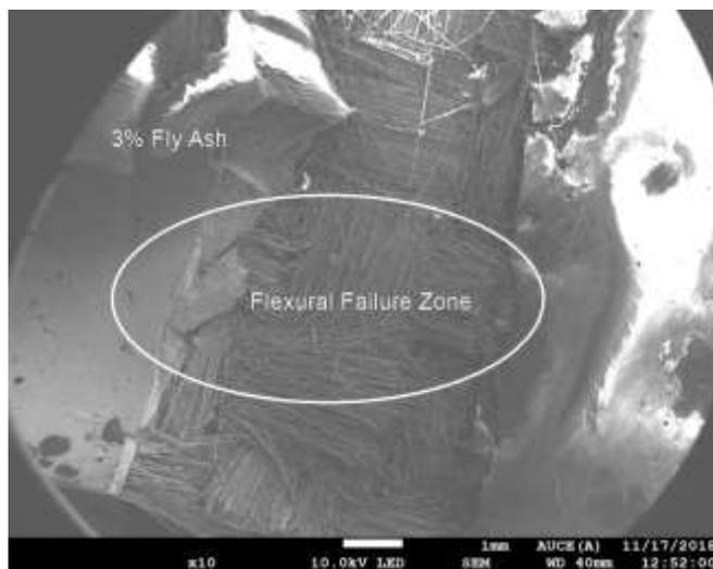
Fig-4: Failure zone of laminate with 3 wt% of Nano fly ash
