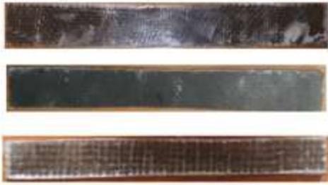
Fig-1: laminates with different wt% of flyash
