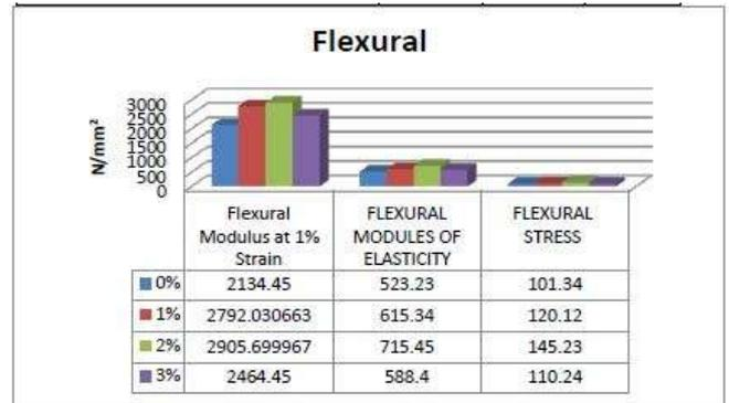
Chart-2: Relation between Flexural Modulus and wt. % of fly ash
