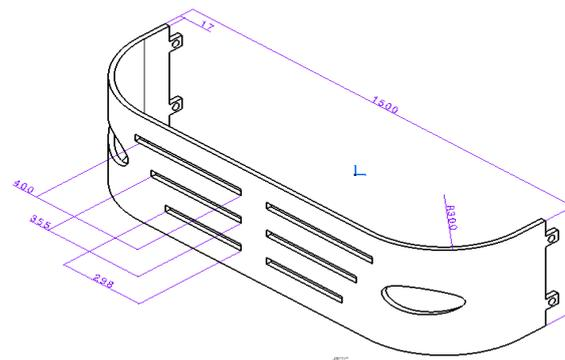
Fig.5 Design of model of bumper in CATIA
