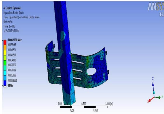
Fig.10 Von Mises Elastic Strain of GFRP
