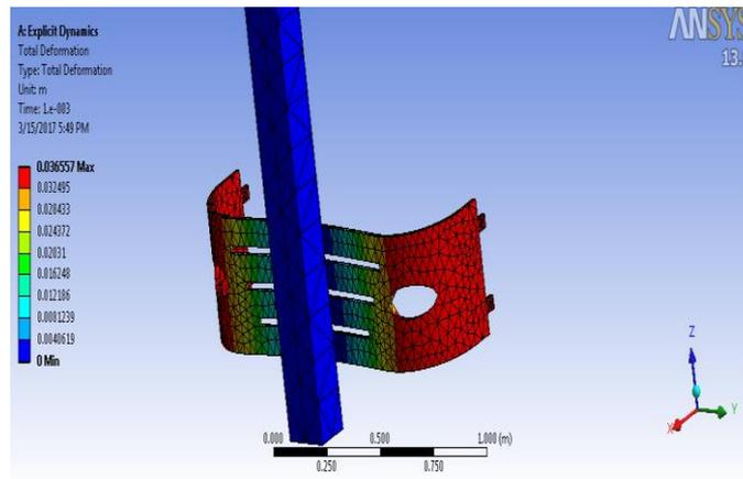
Fig.7 Deformation of GFRP with rubber and wooden powder
