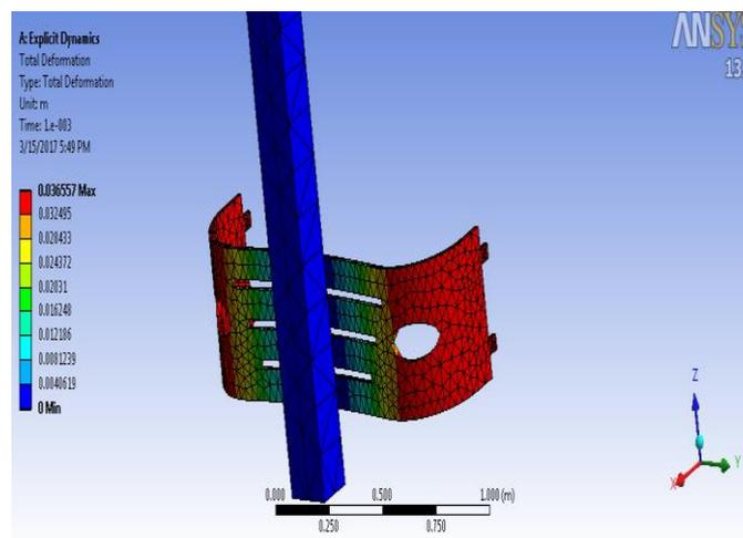
Fig.6 Deformation of GFRP
