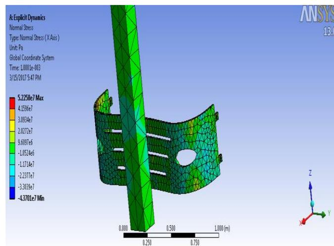
Fig. 9 Normal stress of GFRP with rubber and wooden powder
