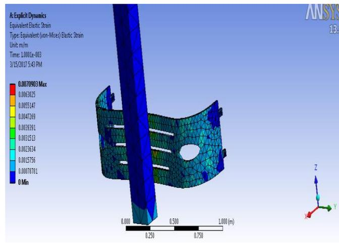
Fig. 11 Von Mises Elastic Strain GFRP with rubber and wooden powder
