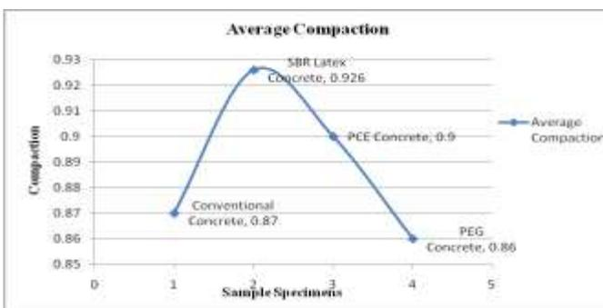
Graph 2: Results of Average Compaction values as observed in test results
