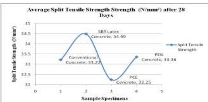
Graph 4: Results of Average Split tensile strength (28 days) as observed in test results
