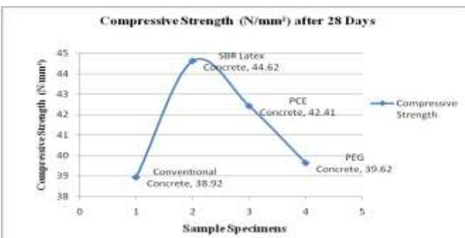
Graph 3: Results of Average Compressive strength (28 days) as observed in test results
