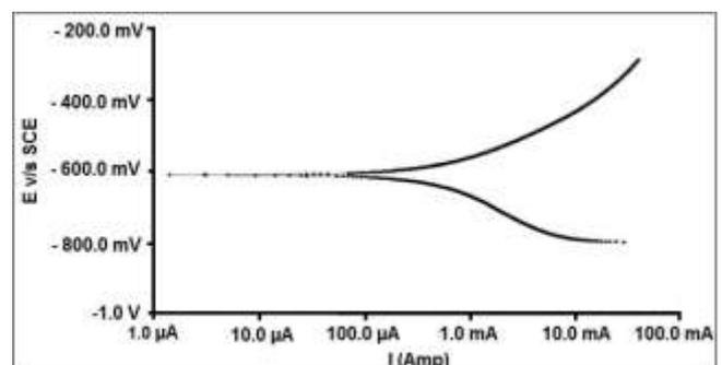
Figure 3: Tafel plot for low carbon steel sample in 3.5 wt% NaCl.
