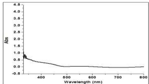
Figure 2: UV-vis scan of conducting poly (aniline-co-o-anisidine) copolymer electrodeposited coating.
