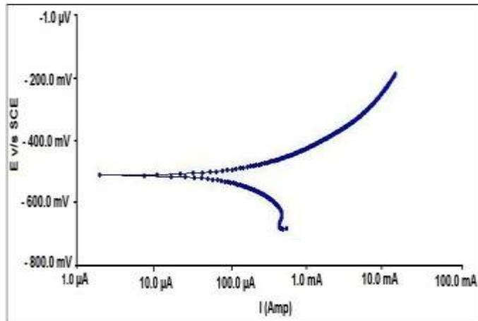
Figure 4: Tafel plot for of electrodeposited conducting co-polymer (0.05M Aniline + 0.05M o-Anisidine) coating on low carbon steel in 3.5 wt % NaCl solution.
