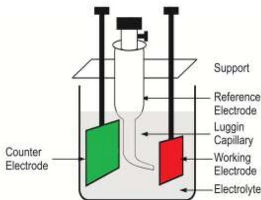
Figure 1: Electrochemical Cell: A line diagram
