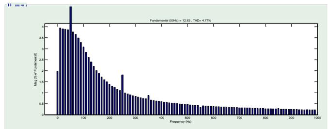
Fig. 5: THD spectrum of Source Current of phase- C with PID controller
