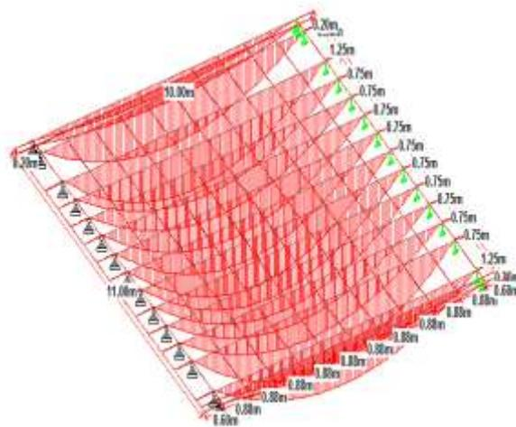
**Figure 8: BM due to 70R tracked vehicle placed on Reinforced concrete slab**
