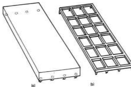
Figure 2: (a) Prototype deck slab model and (b) equivalent grillage model (Source: Bridge Deck Behavior - E.C.Hambly)
