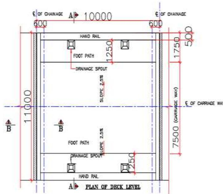
Figure 3: Plan view of Reinforced concrete solid slab
