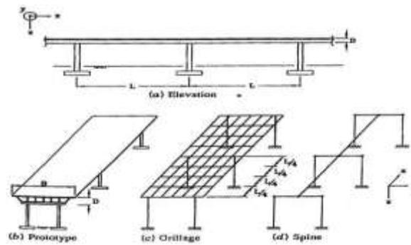
Figure 1: models of super structure (Priestley, et al 1996)
