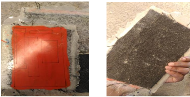
Fig 4. Prepared by using open Mould
