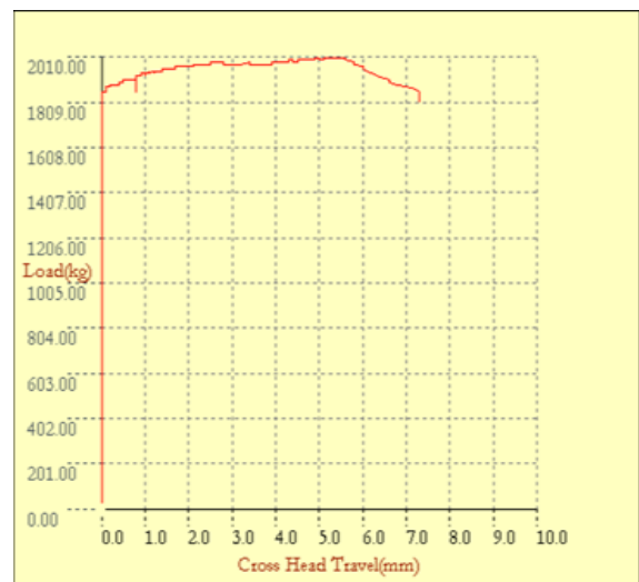
B.3 layers of Sheep wool and 2 layers of E-glass
