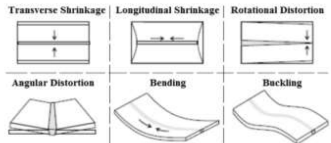
Fig-1: Types of weld distortion
