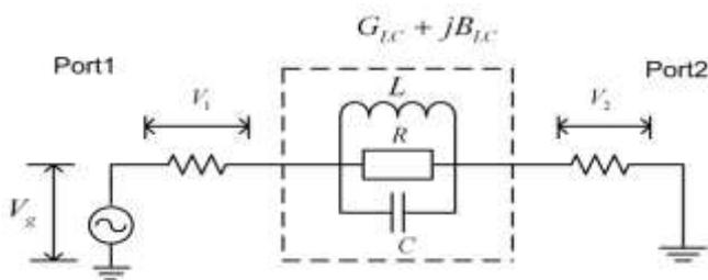
Fig -8: RLC equivalent circuit
