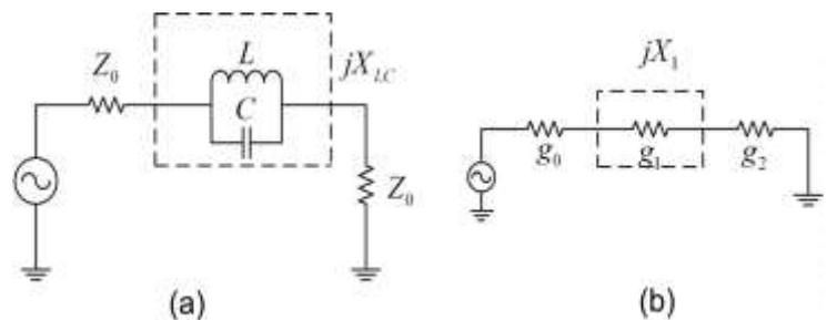
Fig -7: *LC* equivalent circuit: (a) equivalent circuit of the dumbbell DGS circuit,
