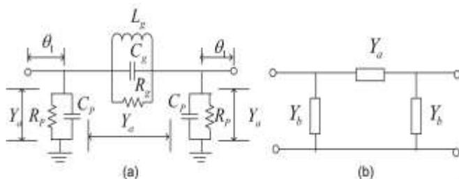
Fig -9:  $\pi$  shaped equivalent circuit for unit DGS: (a) equivalent circuit, (b)  $\pi$  shaped circuit.
