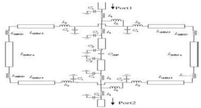
Fig -10:Equivalent-circuit model of unit cell DGS
