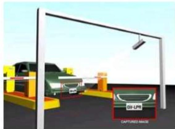
Figure 1: Number Plate detection using image processing
