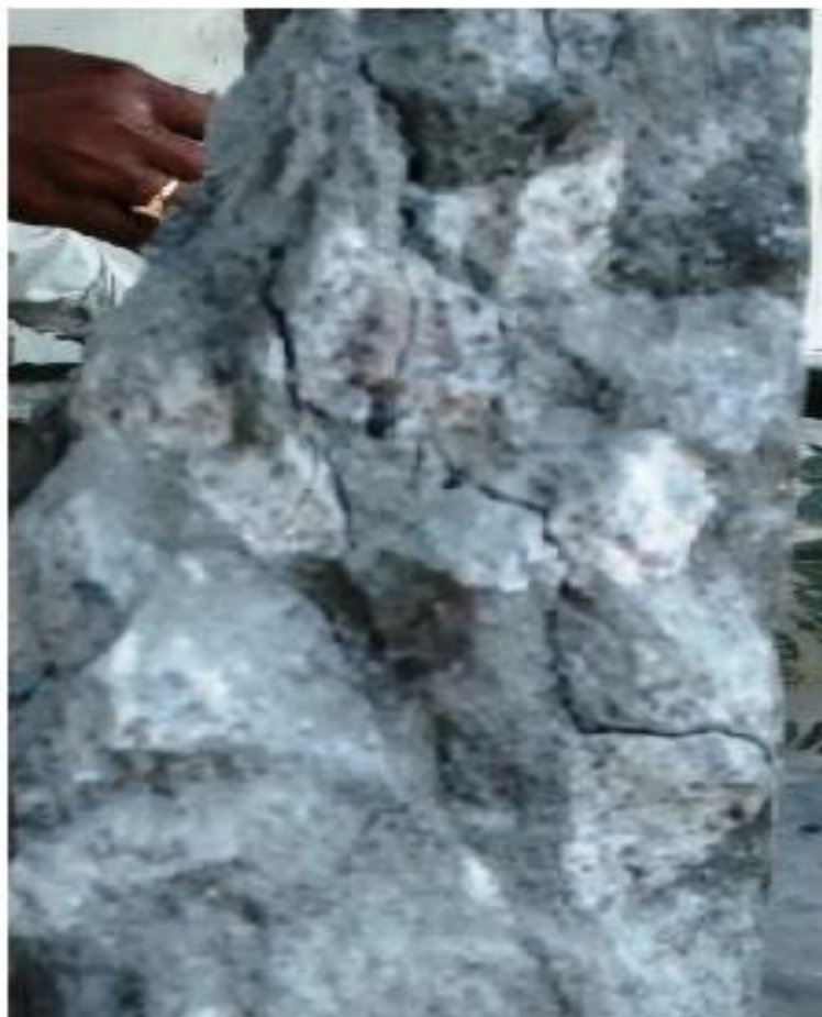
Figure 8. Failure pattern of special concrete
