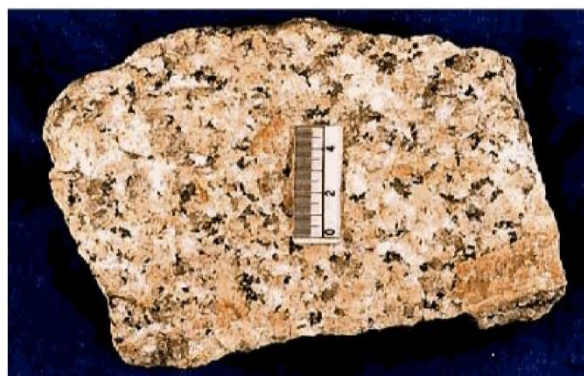
Figure 1. Weathered Coarse Aggregate Sample
