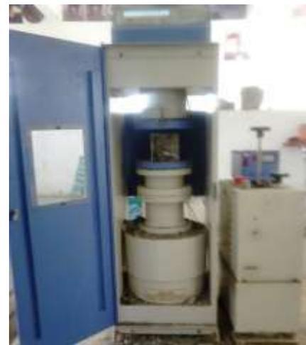
Fig -5: Testing of Concrete Specimen
