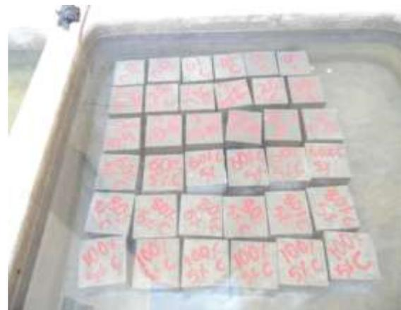
**Fig -3:** Curing of Concrete Specimens in Water
