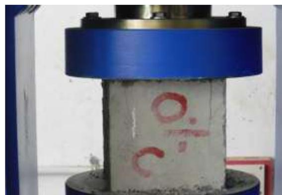
Fig -6: Failure of Concrete Specimen
