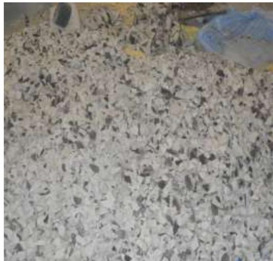
**Fig -1:** Crushed Ceramic Waste
