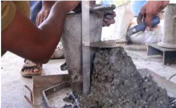
Fig -4: Measurement of Slump
