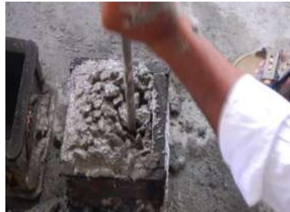
**Fig -2:** Casting of Cube Moulds
