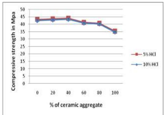
**Graph -3:** Comparison of 28 Days compressive strength for 5% and 10% HCl
