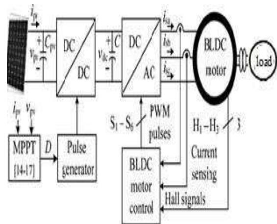
Fig -1: Conventional SPV-fed BLDC motor-driven load
