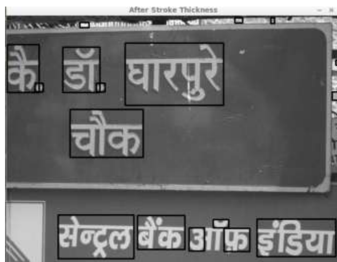
Fig -7: Detection based on headline and vertical line.
