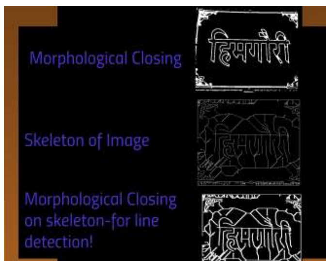
Fig -6: Morphological closing, skeleton of image and morphological closing on skeleton for line detection.
