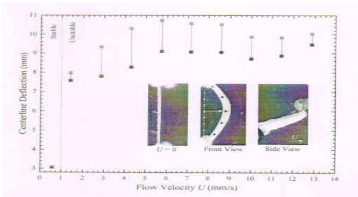
Figure: 3 Bifurcation diagram of the center line deflection of the flexible sheet versus the flow velocity
