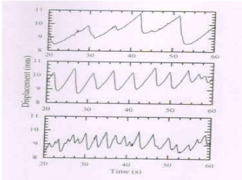
Figure: 4 Time histories of the center line deflection of the flexible sheet at (a)  $U = 4.3mm/s$ . (b)  $U = 7.15mm/s$ , and (c)  $U = 11.44mm/s$
