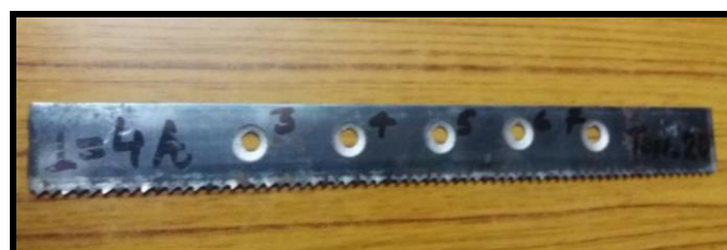
Fig-3: SK2MCr4 carbon tool steel used for experiment for T_{on} (20 \mu s )
