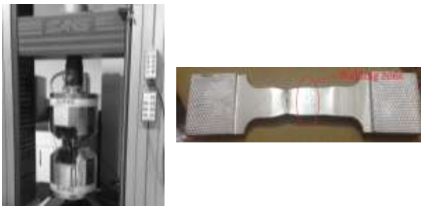
Fig 2-3: Tension test machine, and tested specimen
