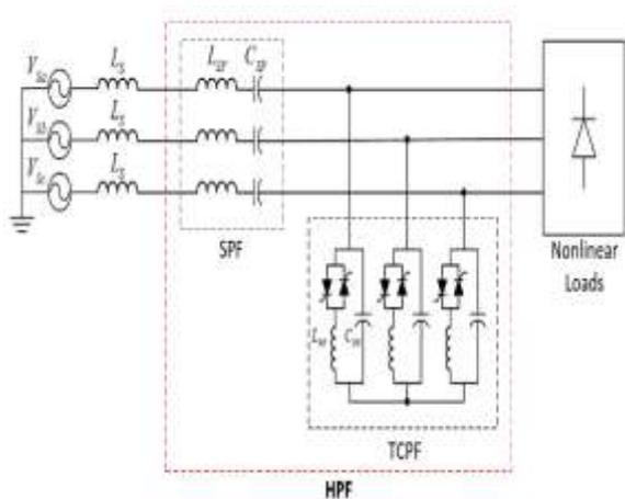
Fig.3 Configuration of the hybrid power filter
