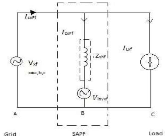
Fig.5 Fundamental equivalent circuit of the proposed APF system
