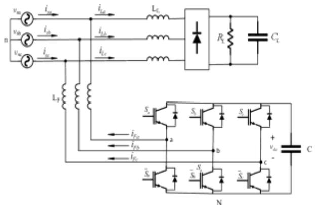
Fig.1 Three phase active power filter
