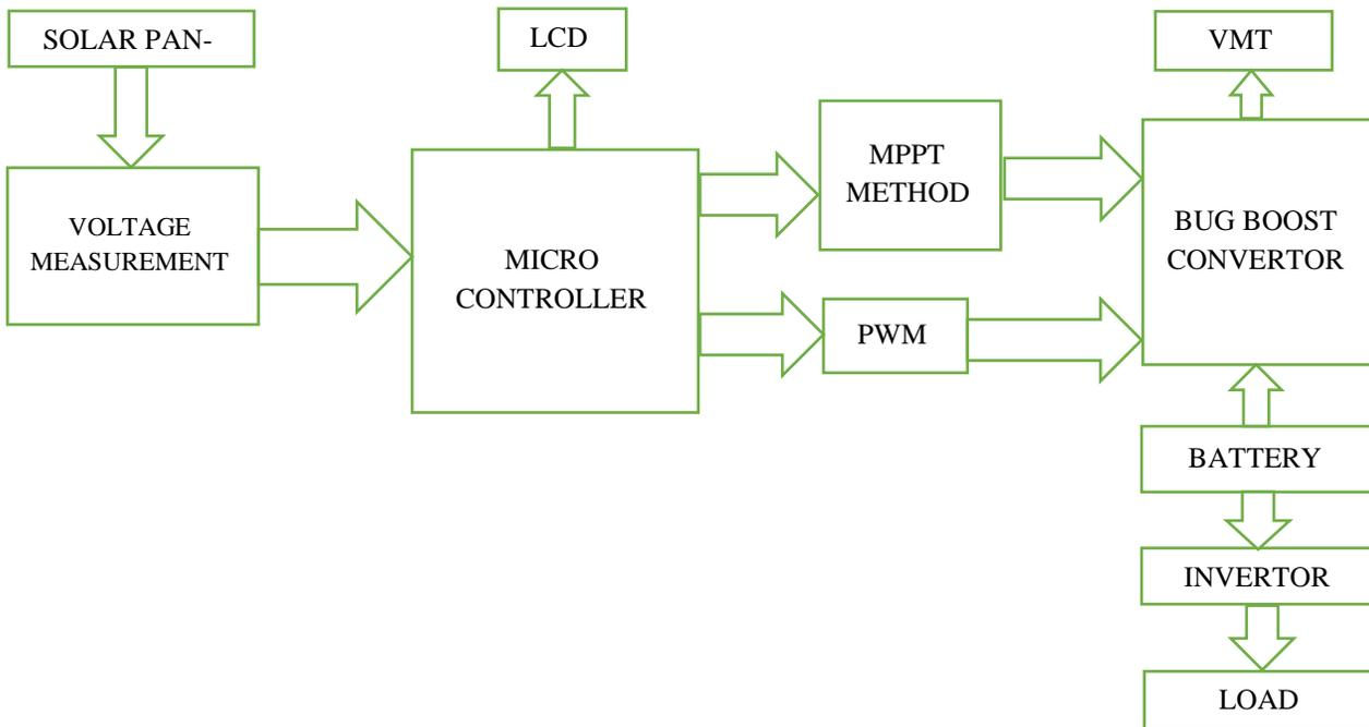
*Figure 1: Schematic of solar power remote monitoring and controlling using IoT*
