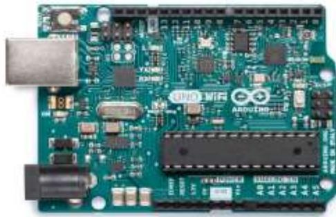
Fig - 2: Arduino UNO development board
