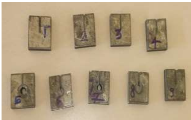
Fig-3: OHNS [E0300] specimen after cut.
