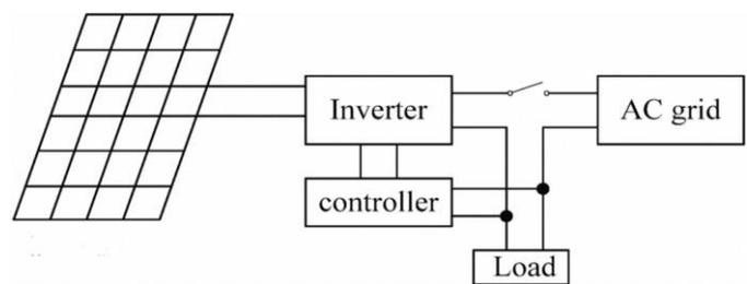
The inverter device with the function of maximum power point tracking can inverse the electric power into sinusoidal current, and connect to the grid. The control system mainly control the maximum power point tracking of photovoltaic, current waveform and power of the output of grid-connected inverter, which makes the output to the grid correspond with the export by PV array.
