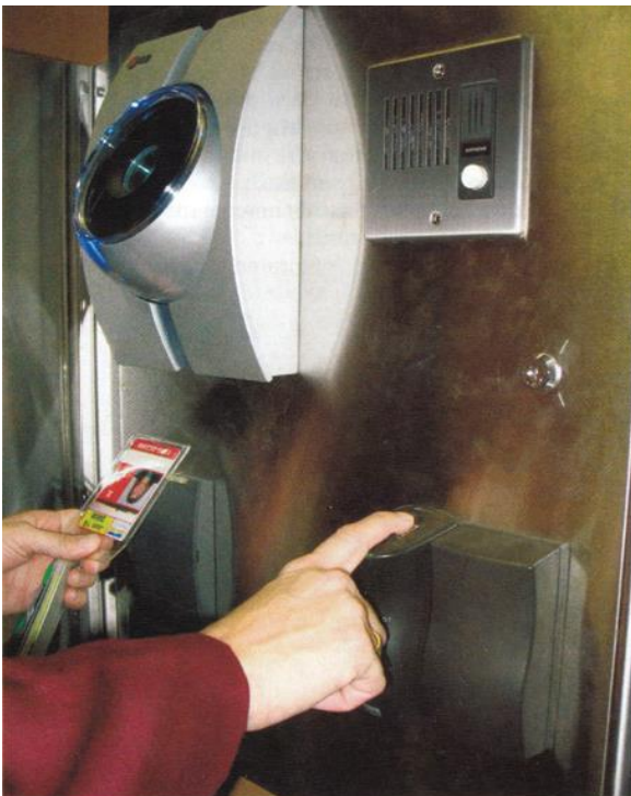
Card swipe and biometrics add essential layers to the setting of Mantrap system
